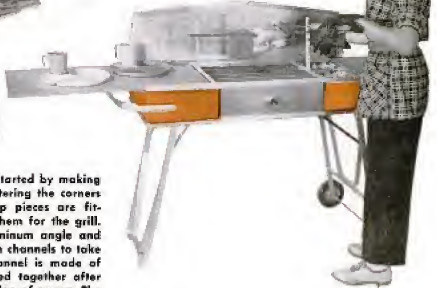
Photo of barbecue, above, shows how the legs appear in the folded position. When the barbecue is set up, ordinary desk-front supports lock legs in place
